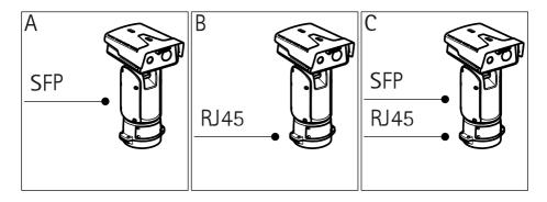
You have different options for installing the network link:
