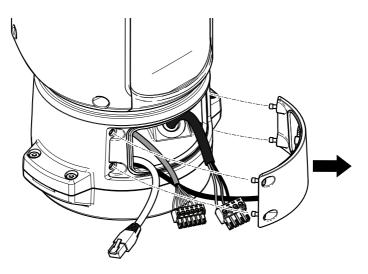
1. Loosen the four lid screws (T20) and remove the lid.
