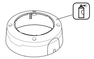
2. Apply a thin and even layer of spray paint according to the instructions of the paint manufacturer.
