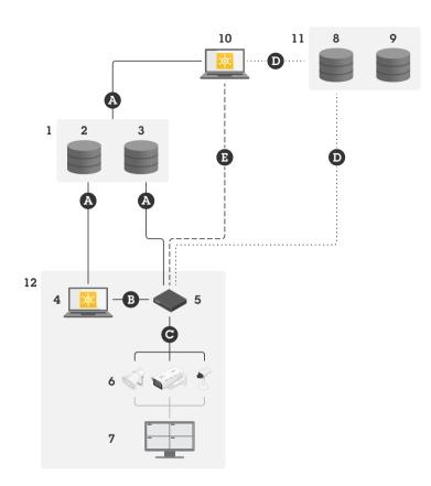
Typical setup for single-site operations with local and remote access.
