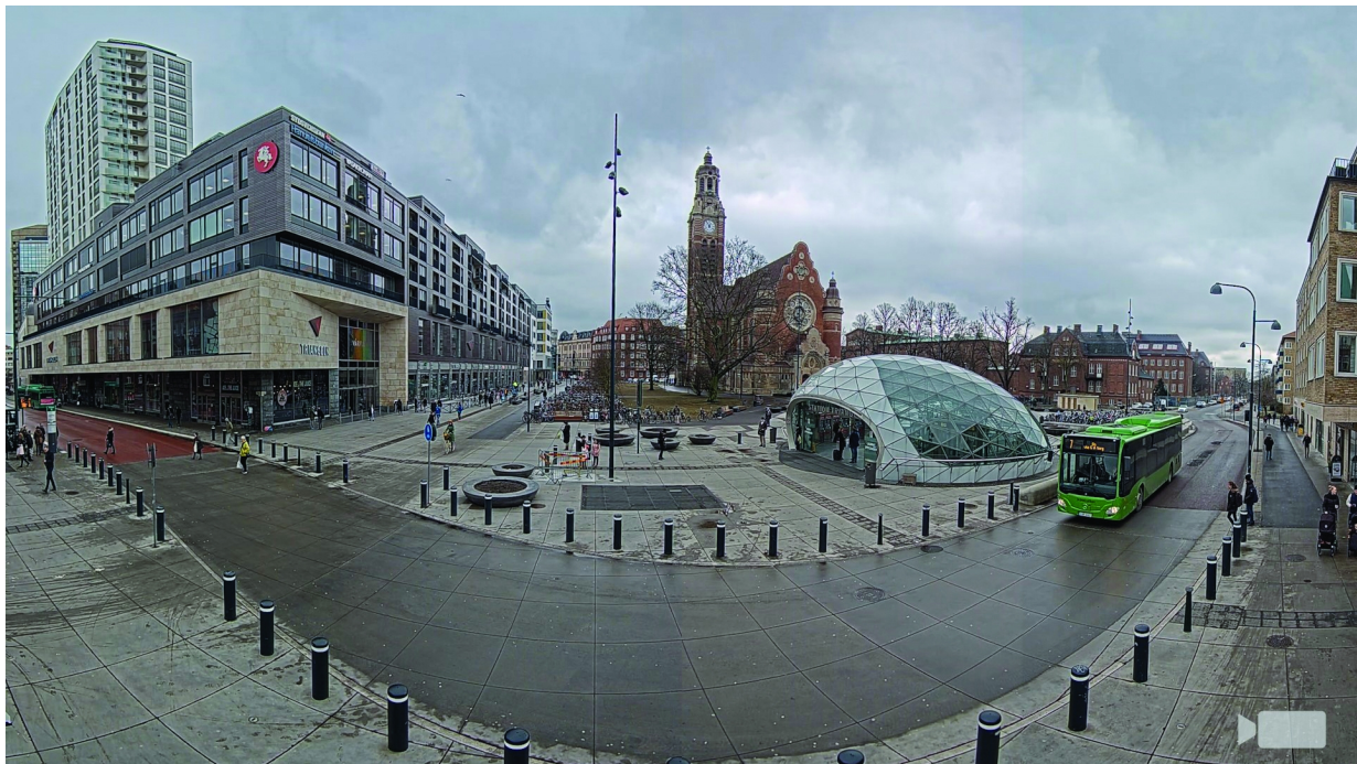
180° view (the street that looks curved is, in fact, straight) from a multisensor camera with four sensors.
