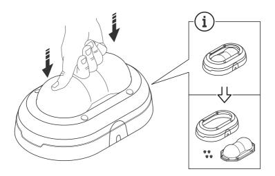
${\it 3.} \quad {\it Use your hand to remove the dome from the dome casing. } {\it Collect the metal inserts.}$
