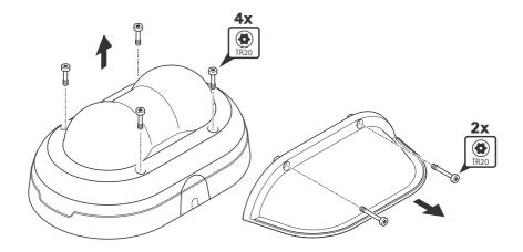
2. Remove the screws from the weathershield (if used) and the dome cover.
