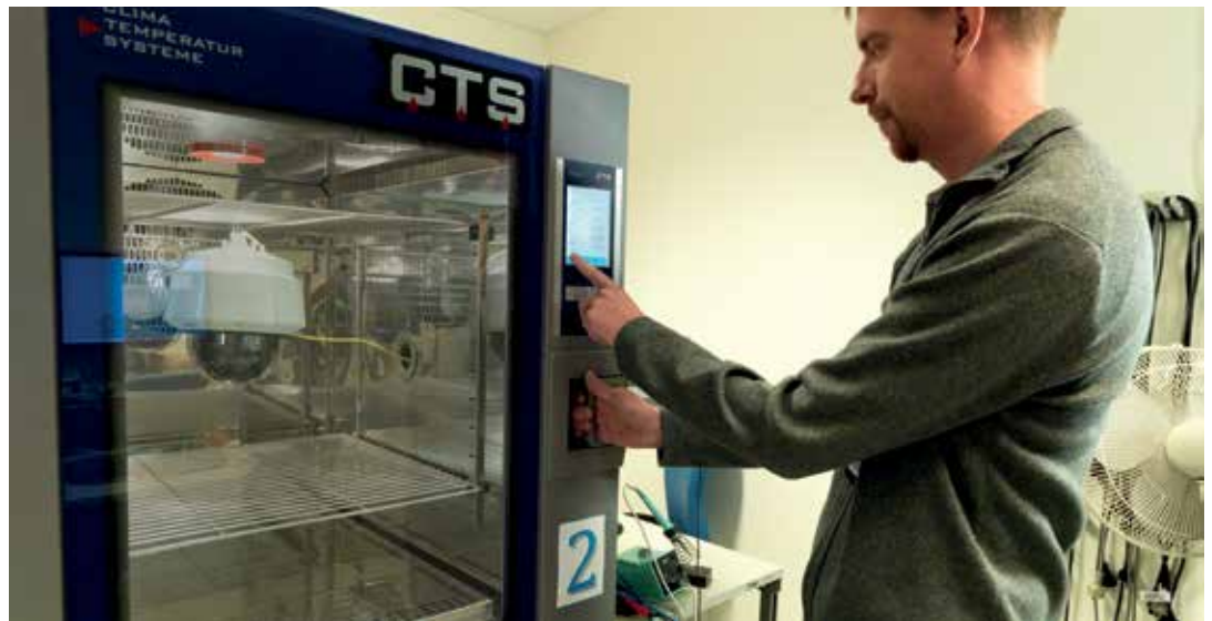
Figure 5: Temperature test in a climate chamber.
