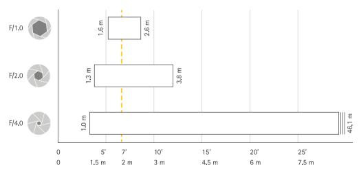
Depth of field examples for different iris sizes with a focal distance of 2 m (7 ft.). A smaller iris opening (that is, a larger f-number), enables objects to be in focus over a longer distance range.
