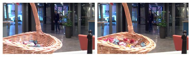
The picture to the left was taken with a camera using a DC-iris lens. The picture to the right was taken with a camera using a P-Iris lens and exhibits a greater depth of field than the picture to the left.
