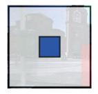
3. Use the **Sensitivity** slidebar to define how sensitive the detection should be. The lower sensitivity selected on the **Sensitivity** bar, the greater difference in luminance is needed between the object and the background for the detector to be activated.
