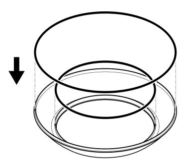
1. Reassemble the two dome ring gaskets.
