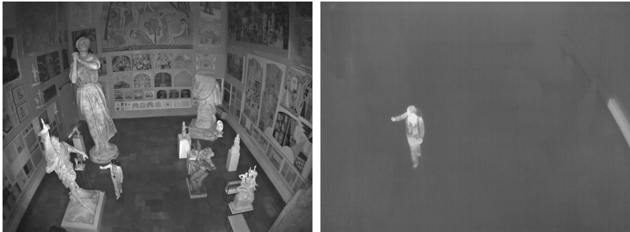
Figure 4. Images comparing day-and-night camera and thermal camera, both captured in darkness.
