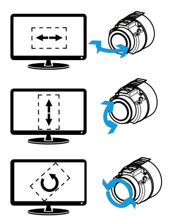
The illustration shows how the directions pan, tilt, and roll affect the live view image.
