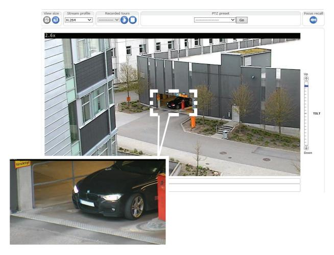
The image shows an example of a focus recall area marked with a white square. As soon as the camera detects the focus recall area, the camera recalls the previously set focus. This means that, in this example, the focus is set on the car regardless of zoom factor.
