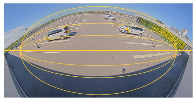
180-degree panoramic view snapshot taken with a multisensor camera without horizon straightening. The lines added on the image give a clue about how the wide-angle multisensor output has been projected to create one, rectangular image. All lines come off as bent or tilted except for the horizontal and vertical center of the view.
