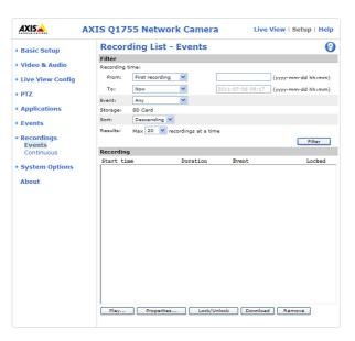
The Network Camera can be set to record continuously or as result of a triggered or scheduled event. See *Continuous Recording, on page 35* and *Event Types, on page 29* for more information. The Recording List window contains a list of recordings made to the local storage. It shows each recording's start time, length, the Event type used to start the recording, and if the recording is locked so that it can neither be deleted nor recorded over.
