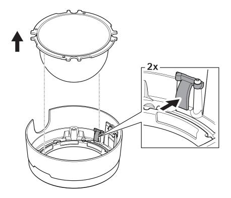
5. Remove the dome from the dome cover by pressing the two spring holders.
