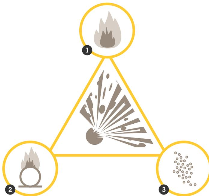
*Three components must be present for an explosion to occur:*
