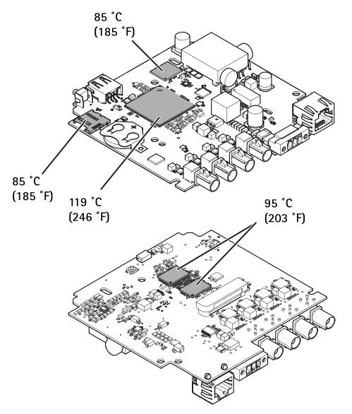
1 Maximum allowable temperatures. If the ambient temperature is 35 °C (95 °F) or higher, the temperature of the components increases and they must be cooled.
