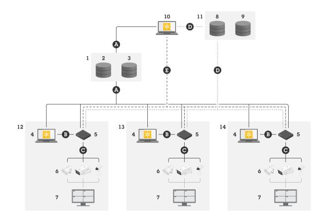
Multisite setup using local and remote access.
