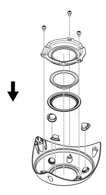
5. Re-tighten (to 2 N m) the three T20 screws that hold the front chassis in place.
