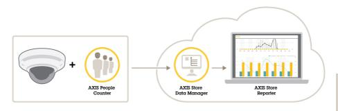
An overview of the different products, applications, and tools needed for a complete system.
