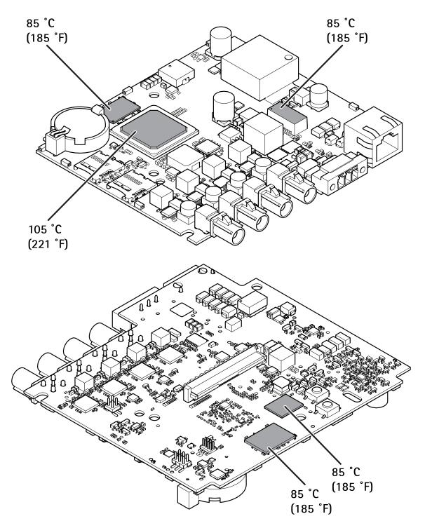
1 Maximum allowable temperatures. If the ambient temperature is 35 °C (95 °F) or higher, the temperature of the components increases and they must be cooled.
