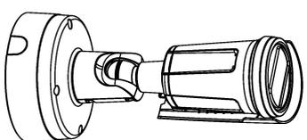
Weather Shield sliding direction: 15.5mm [6.10]
