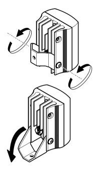
If required, loosen the screws and change to a diverging lens with the desired angle of illumination. The angle of illumination should be adjusted according to the camera field of view to light the whole scene adequately. See *Technical Specifications*.
