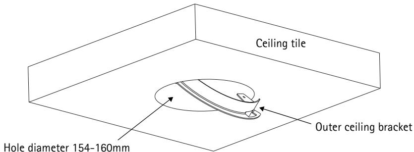
5. Pull all of the required cables (network, power) and the safety wire down through the hole, ready for connection.
