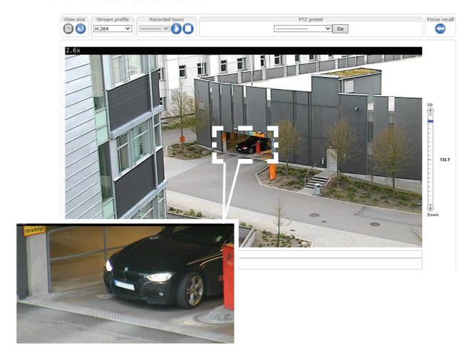
The image shows an example of a focus recall area marked with a white square. As soon as the camera detects the focus recall area, the camera recalls the previously set focus. This means that, in this example, the focus is set on the car regardless of zoom factor.
