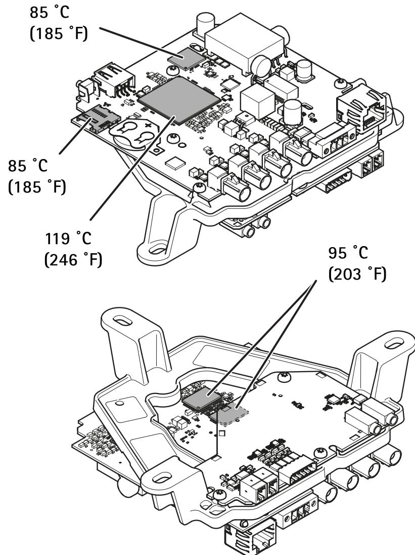
**Maximum allowable temperatures. If the ambient temperature is 35 °C (95 °F) or higher, the temperature of the components increases and they must be cooled.**
