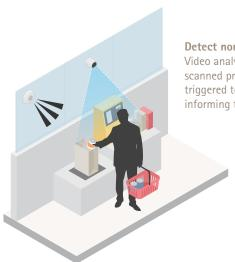
Detect non-scans at self-checkouts Video analytics can detect nonscanned products and audio is triggered to play a voice message informing the customer.
