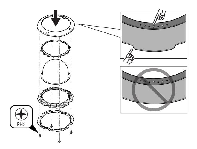
3. Assemble the dome module bracket, dome with dome module sealing and dome cover ring (4 screws, 1.2 N m).
