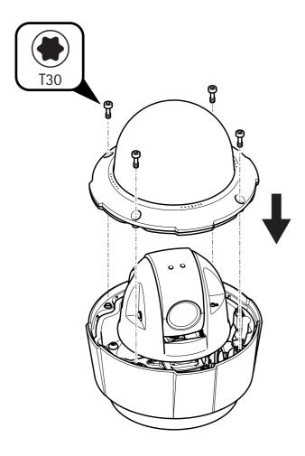
4. Reassemble the dome module assembly (4 screws, 4 N m).
