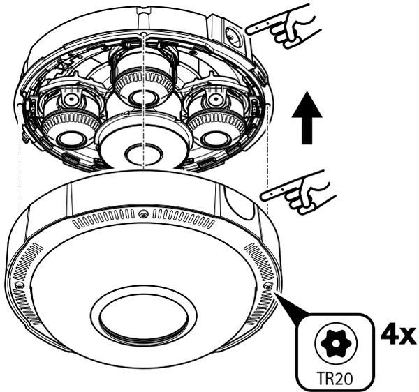
3. Reassemble the dome cover and the camera unit and tighten the screws (torque 1.0 Nm, 0.7 lb ft).
