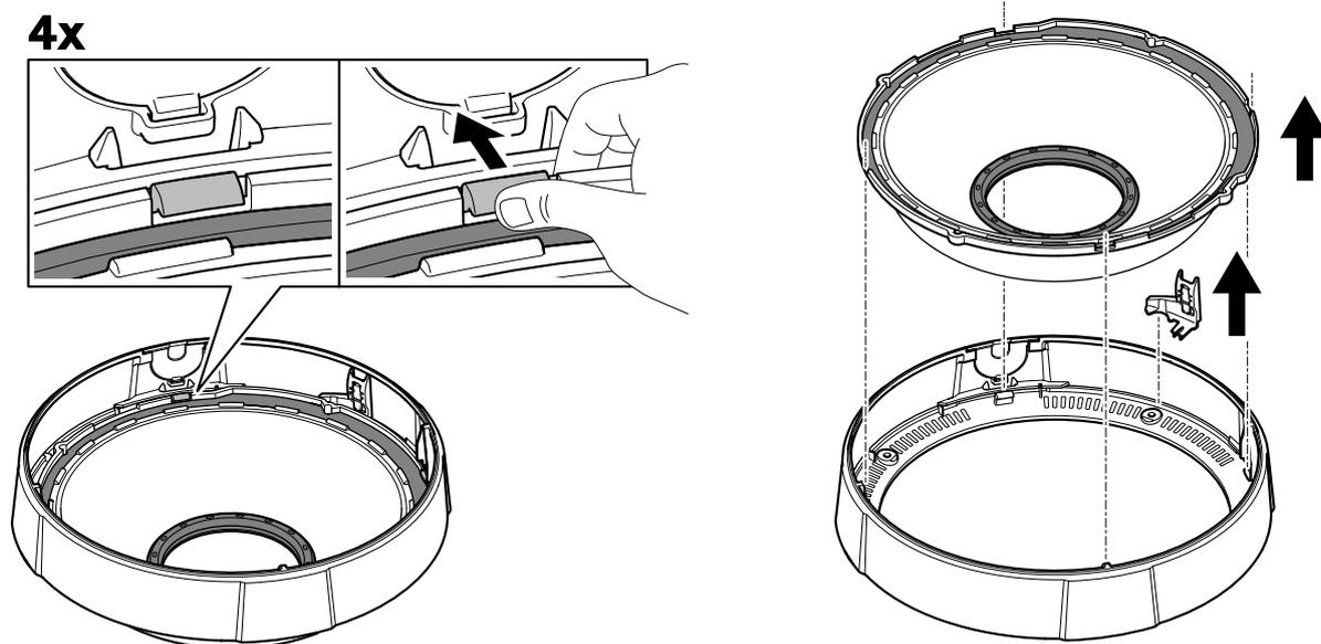
3. Remove the dome and the plastic holder from the dome cover.
