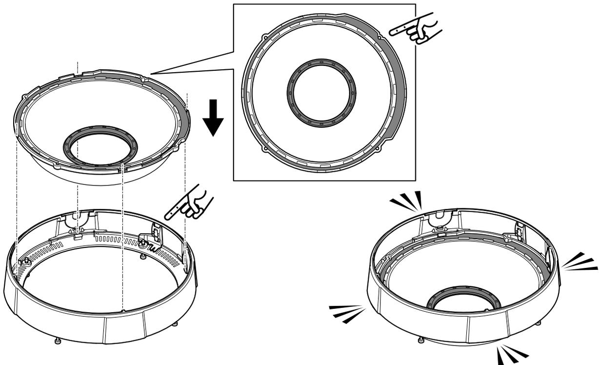
2. Line up the dome to the dome cover as shown in the image and snap the two parts together (4 snaps).
