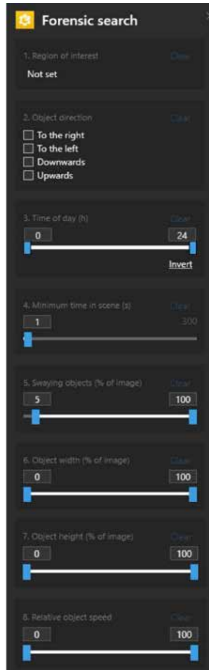
Range of metadata attributes sent from Axis devices used to match search queries
