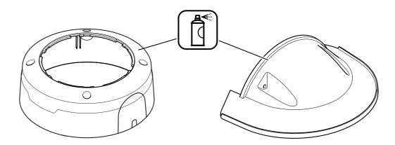
2. Apply a thin and even layer of spray paint according to the instructions of the paint manufacturer.
