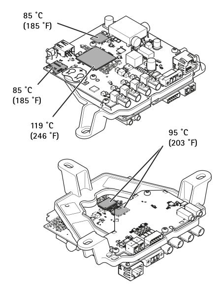
Maximum allowable temperatures. If the ambient temperature is 35 °C (95 °F) or higher, the temperature of the components increases and they must be cooled.
