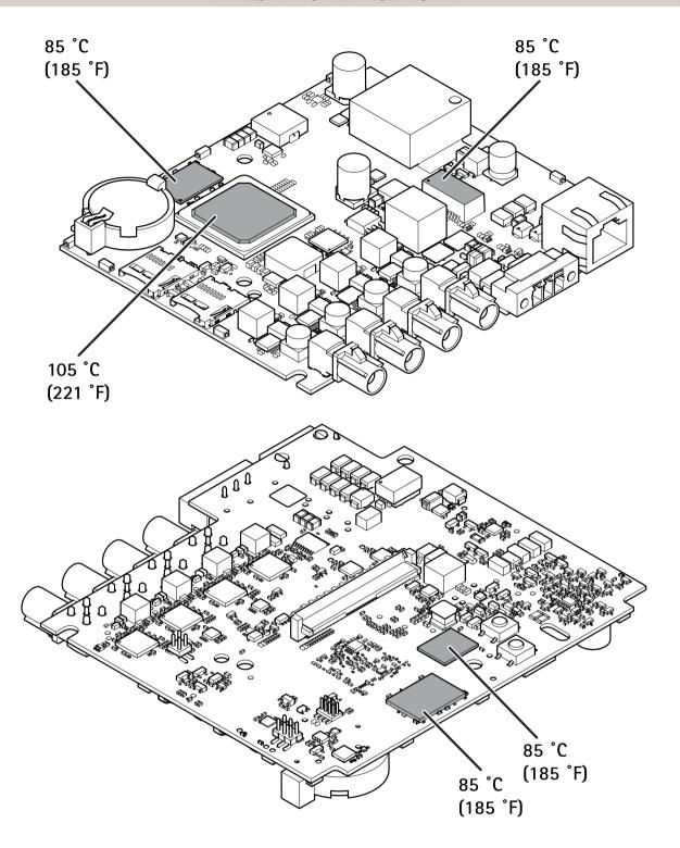
Maximum allowable temperatures. If the ambient temperature is 35 °C (95 °F) or higher, the temperature of the components increases and they must be cooled.
