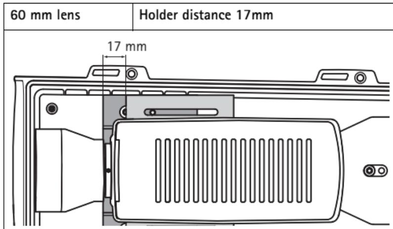
3. Measure the holder distance on both sides of the camera to make sure the camera and holders are mounted parallel to each other.
