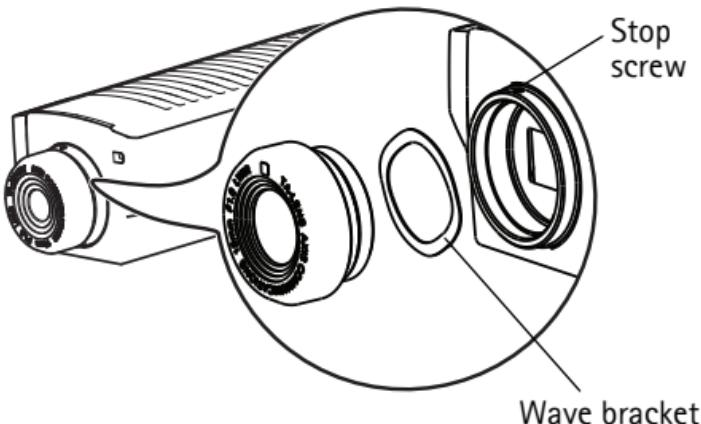
3. Unscrew the lens by turning it counter-clockwise.
