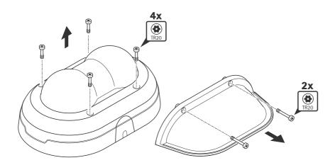
2. Remove the screws from the weathershield (if used) and the dome cover.
