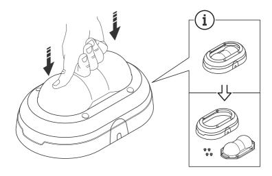
3. Use your hand to remove the dome from the dome casing. Collect the metal inserts.
