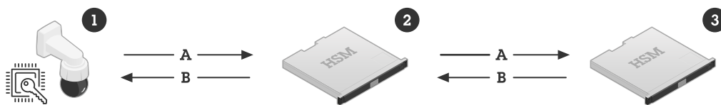
Figure 2. Axis IEEE 802.1AR public-key infrastructure (PKI) for factory-provisioning the Axis device ID during the manufacturing process. Axis device ID (1), which is a certificate incorporating the serial number of the product, is signed by an Axis device ID intermediate CA (2), which was signed by the Axis device ID root CA (3). Dedicated hardware security modules (HSM) are used for secure factory provisioning.
