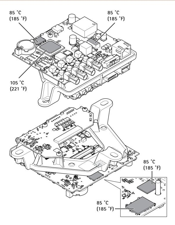
1 Maximum allowable temperatures. If the ambient temperature is 35 °C (95 °F) or higher, the temperature of the components increases and they must be cooled.
