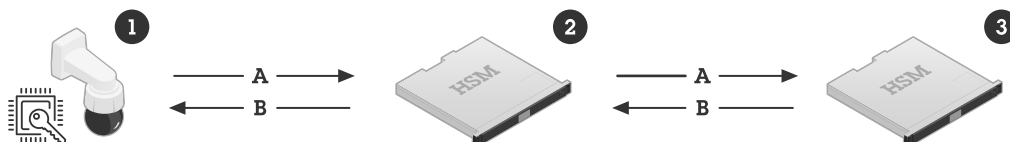
Figure 5. Axis IEEE 802.1AR public-key infrastructure (PKI) for factory provisioning the Axis device ID during the manufacturing process. Axis device ID (1), which is a certificate incorporating the serial number of the product, is signed by an Axis device ID intermediate CA (2), which was signed by the Axis device ID root CA (3). Dedicated hardware security modules (HSM) are used for secure factory provisioning.
