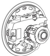
4. Attach the dome cover and secure it by tightening the captive screws.
