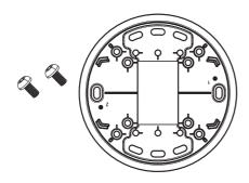
Thread the necessary cables through the bracket.
