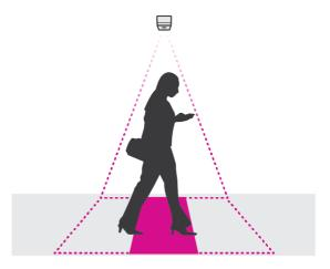
• Make sure the camera is facing straight down, in line with the ceiling.
