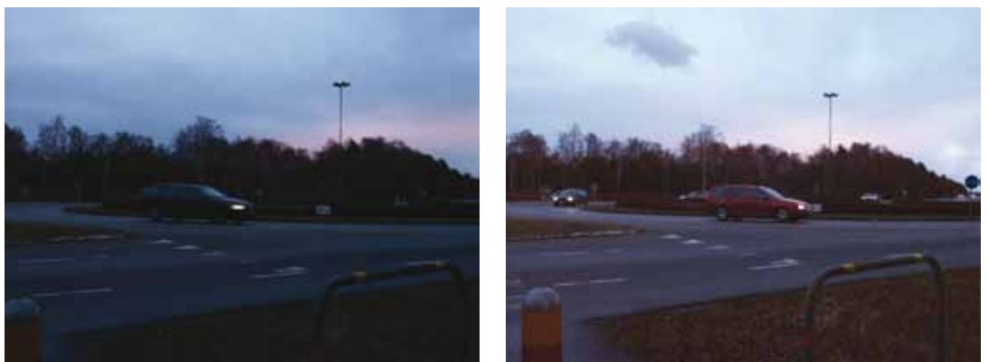
Figure 3. At left, a scene taken at 500 lux with low gain. At right, a similar scene also taken at 500 lux but with high gain. The images illustrate how an increase of the gain will amplify the video signal and make the image brighter at the sacrifice of increased noise in the image.
