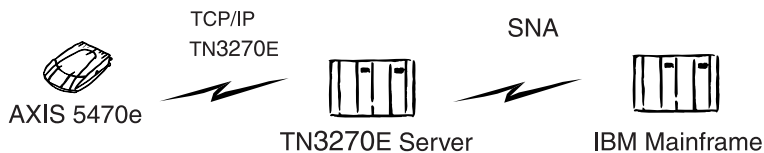
Typical AXIS 5470e TCP/IP TN3270E Network Configuration
