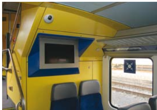
The AXIS 209 Network Cameras measure only 4 cm (1.5 in.) high and 10 cm (4 in.) wide. Their compact, discreet design and rounded edges make them ideal for onboard mounting in ceilings or on walls.
