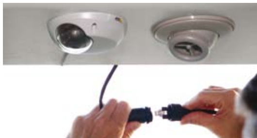
One cable is all it takes when installing an onboard network camera, eliminating the need for a separate power cable. The connector types used, e.g. M12 or Woodhead, are suitable for mobile transportation.
