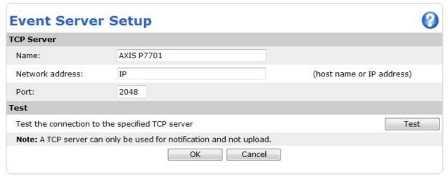
Figure 6. Setting up an event server in AXIS P8221. Replace "IP" with the IP address of AXIS P7701.
