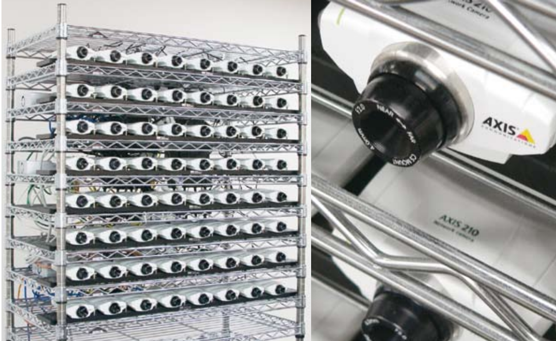
Real-time system for image-based rendering from a multi-view video, consisting of a total of 64 video cameras.
