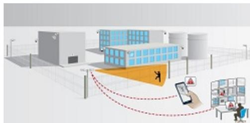
Combined with network cameras, network horn speakers and video management software, AXIS Perimeter Defender forms a comprehensive, video-based solution for effective perimeter surveillance and protection
