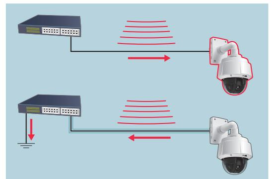
For this to work, it is imperative that the **PSE is properly grounded**. An Axis PoE midspan should **always be connected to a grounded socket** for the shield to function properly.
