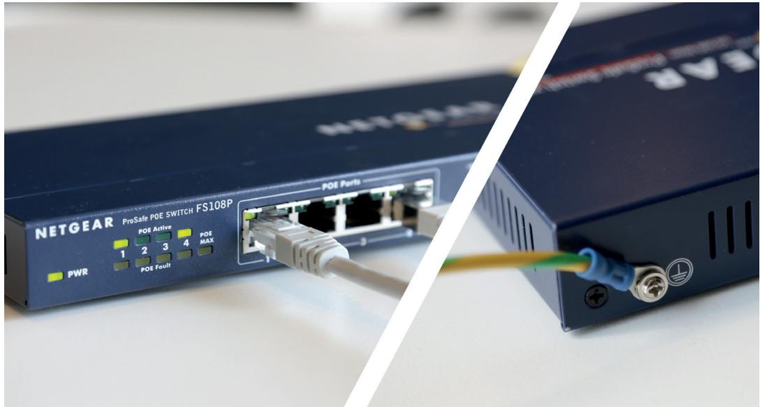
However, a desktop switch like the one shown in the image above may lack a ground connection through the power line; therefore, the switch **needs to be grounded separately**.
