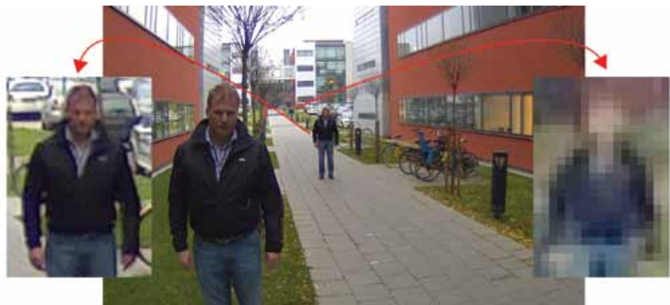
Figure 5. In the main image the three operational requirement criteria. Enlargement of Recognition (Left) and Detection (Right).
