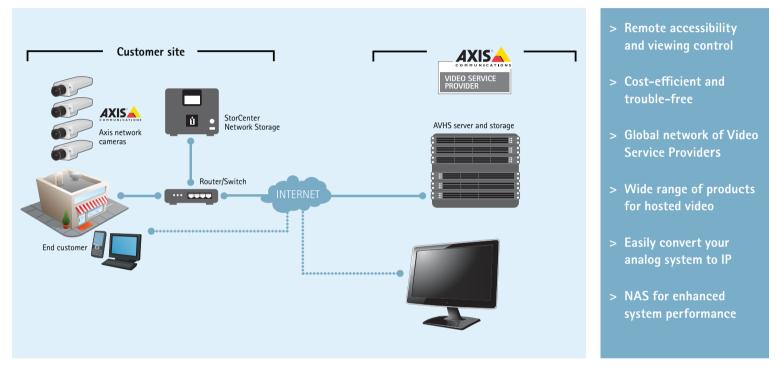
An Axis network camera with support for AXIS Video Hosting System (AVHS) allows end customers using a video hosting solution to view an area and access the system from anywhere and anytime, as long as an Internet connection is available. At work, at home or on the road – you can log in to the service portal from a PC, laptop or most modern cell phones.
