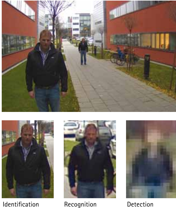
Figure 2. The different resolutions for Identification, Recognition and Detection.
